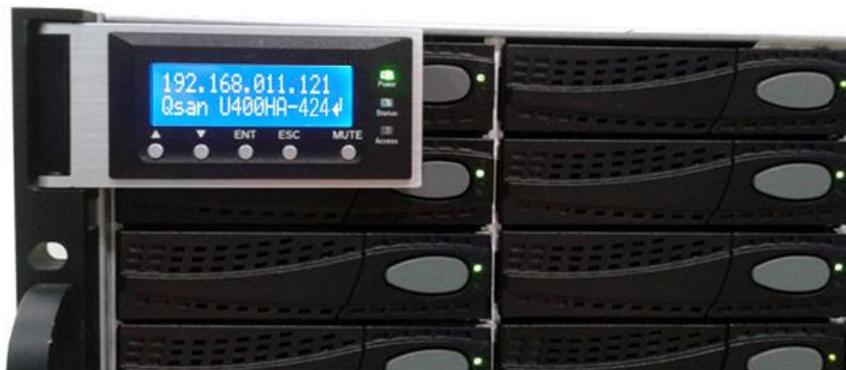
Fig 1-1 LCM display (IP address)
